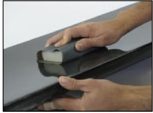
Figure 6. Block sanding the wing to remove any surface imperfections.
