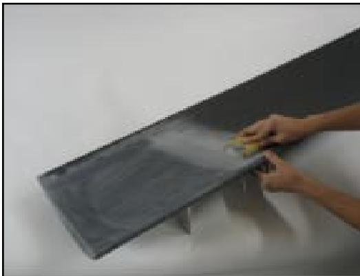
Figure 23. Because of the heavy print through and surface scratching, this wing is first being block sanded with 80 grit, dry sandpaper.
