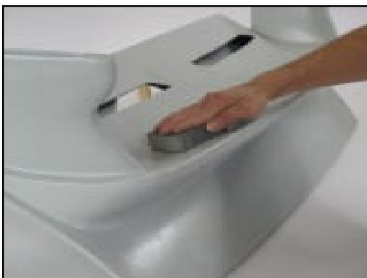
Figure 21. Block sanding so that the last primer can be applied.
