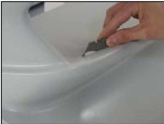
Figure 20. Filling in small imperfections with body filler.
