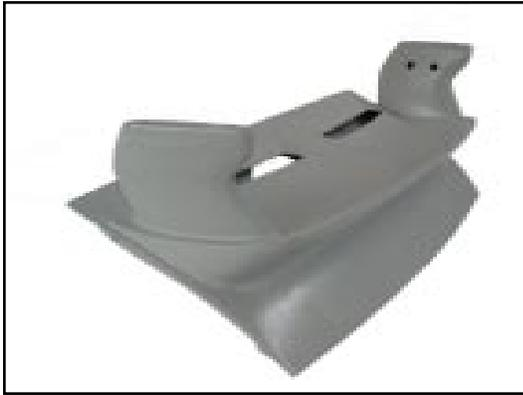
Figure 19. A primed composite tailbase, ready for preparation. If you are starting with a gel coated part, please refer to FRP TECHNIQUES for the correct additional steps required to reach the primer stage.
