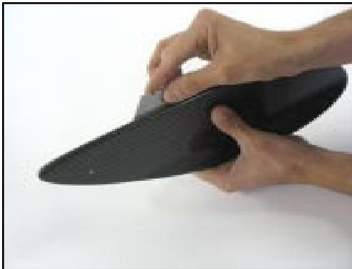
Figure 12. Your first step is to repair any imperfections. Here, the paint technician is using a razor blade to spread some body filler in small pin holes.
