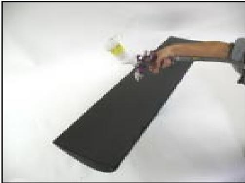
Figure 17. Spraying the entire wing with a high quality clear coat.
