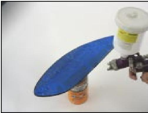
Figure 15. The trim line being sprayed black.
