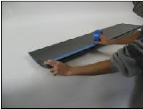
Figure 7. Masking off for painting the trim lines.
