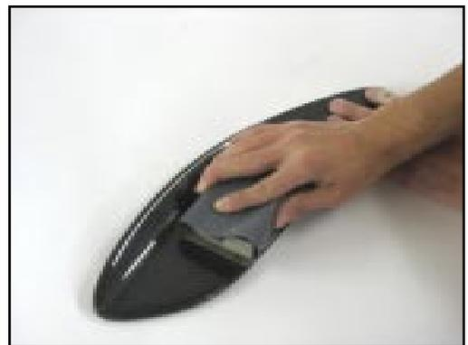
Figure 13. Next, the end plate is block sanded.
