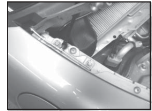
PHOTO 6 The hinge mounting bolts. For aligning the hood to the fender.
