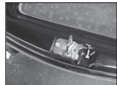
PHOTO 8 Installing the front hatch.
