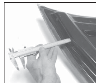
PHOTO 2 Checking for correct bolt length.
