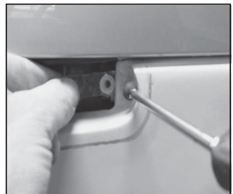
PHOTO 11 Wrapping the washers in a piece of tape will make it easier to slide them into place.
