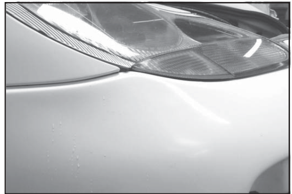
PHOTO 14 After slipping the new bumper in place, and reinstalling the head lights see how the corner at the head light lines up.
