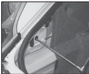
PHOTO 2 Removing the head lights Passenger side- Clockwise off Counter Clockwise on Driver Side- Counter Clockwise off Clockwise on
