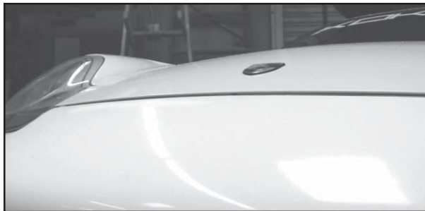
Photo 15 Correct alignment on the hood seam.
