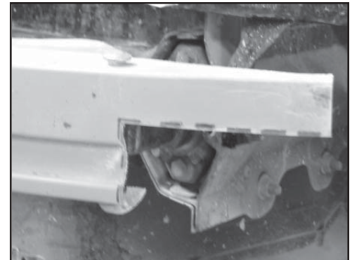
Photo 15 The blade reinstalled after it's been notched
