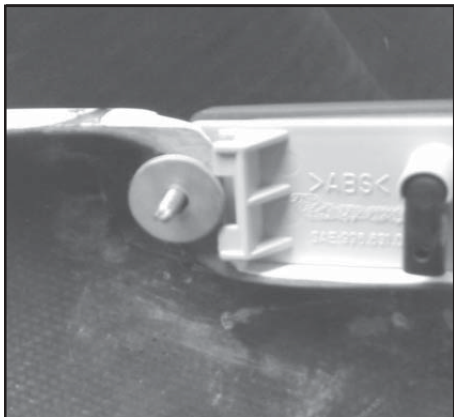
PHOTO 12 These two small washers will provide a space for the tabs on the light to fit behind.
