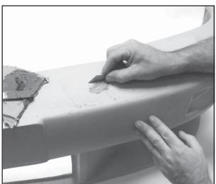
PHOTO 13 Pin Holes Imediately after the first primer drys check the surface for pin holes and use a razor blade to spread fill in them.
