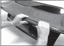
PHOTO 12 Squeeze all the seams and thin edges to check for open edges.
