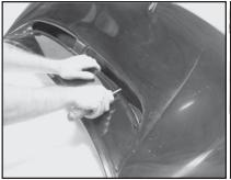
PHOTO 11 Checking for air Using the round shaft of a screwdriver rub hard on all the edges and corners.
