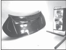
PHOTO 10 Post Curing Here a small heat lamp is being used to cure this 996 ERS tailbase.
