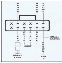
**PHOTO 15** The MPC for model years 99,00,01, with third brake light.
