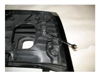
6. Remove the 4 bolts from the hinge holding the plastic tray to the front of the decklid.
