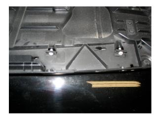
4. Remove the press on clips that hold the support rail securing the bottom of the bellows.
