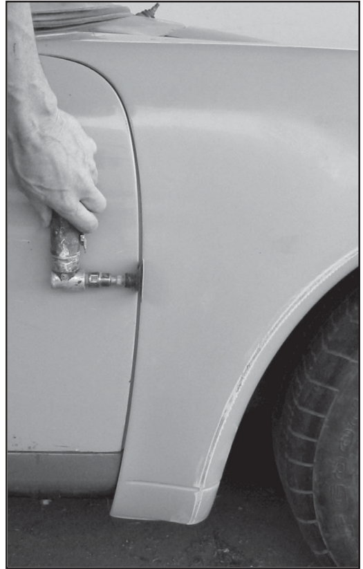
PHOTO 15 Grinding the seam. Use a right angle die grinder with an #80 grit disc. You may need to relieve the inside corner also so the door doesn't catch when opening.
