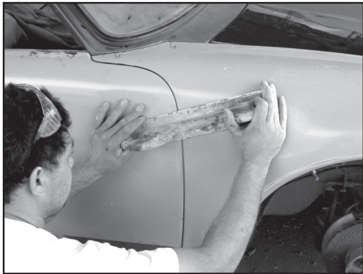
PHOTO 17 Block sanding across the door and fender for a perfect match.
