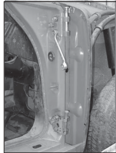
PHOTO #7 Installing the hinge halves onto the front lockpost
