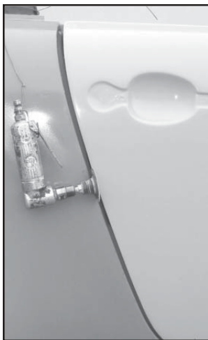
PHOTO 10 Use an angle grinder to make the seam even. This door can probably be spaced back to tighten the gap.
