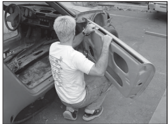
PHOTO #8 Hanging doors is a one man job.
