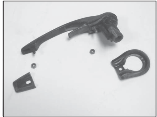
PHOTO 12 The door handle, mounting nuts and gaskets
