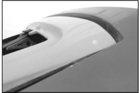
Photo 12 Top Low Too many washers at the rear bolt.
