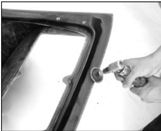
PHOTO 9 Grinding the bottom corner so it clears and won't scuff on the edge of the window frame.
