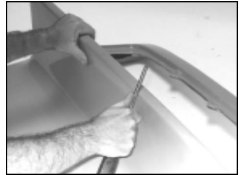
PHOTO 21 Checking for air bubbles.
