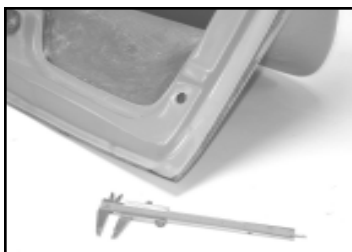
PHOTO 5 Drill hole for the snubber
