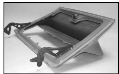
PHOTO 7 Hinges and Plunger installed
