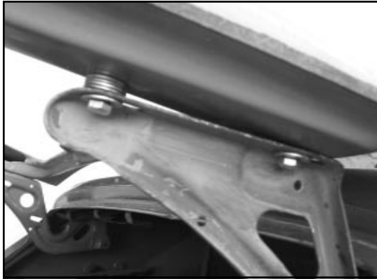
PHOTO 11 Rear Washer Stack Place washers here to lower the front edge.
